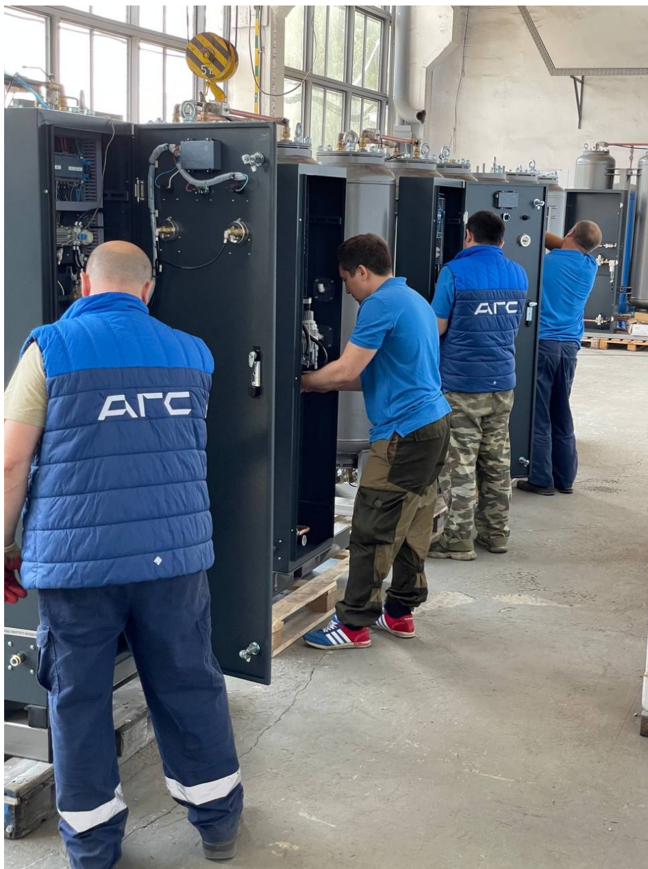
Assembly of serial generators
